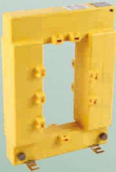
MODEL-VIPS SC03 Primary : 500A to 1500 Secondary : 5A / 1A Bus Bar Dimension : 80 (H) x 120 (W)
