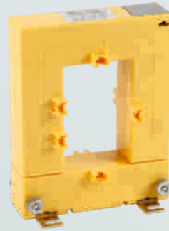
MODEL-VIPS SC02 Primary : 250A to 1000 Secondary : 5A / 1A Bus Bar Dimension : 50 (H) x 80 (W)
